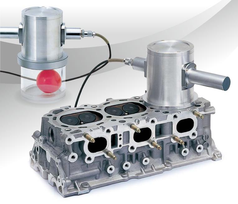
• Acoustical Capacity Meter (Combustion Chamber Capacity Meter)
